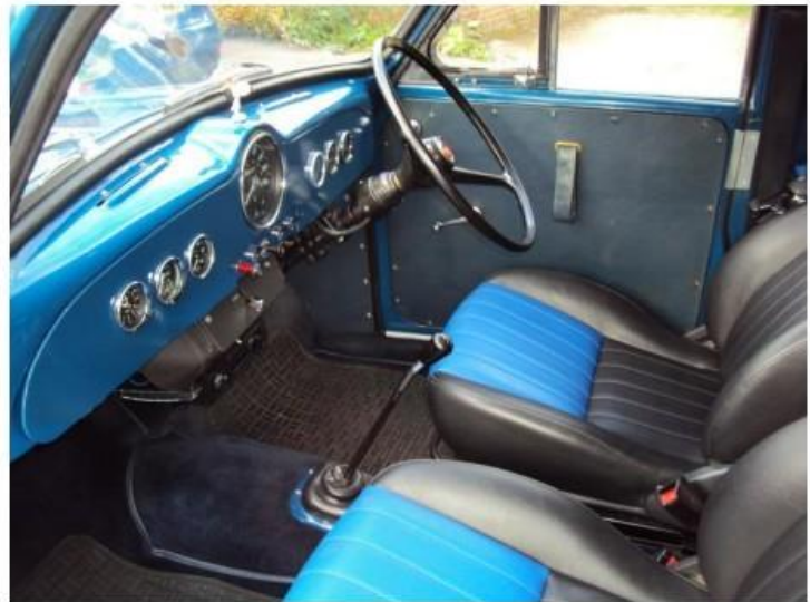
A view of the current interior showing the modified dash with hinged, drop-down panels for the gauges and Metro seats.
