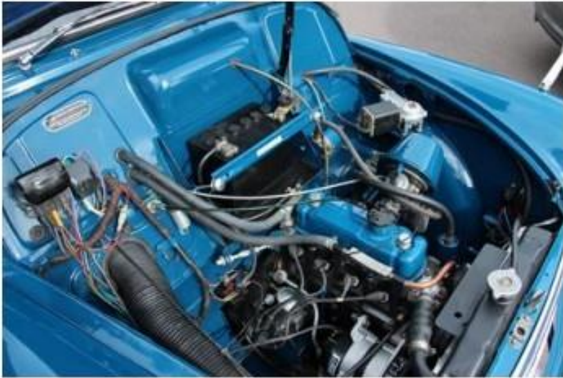
Looking very smart now with fresh paint and a new 1275 along with a Midget Clutch and extended clutch release arm.
