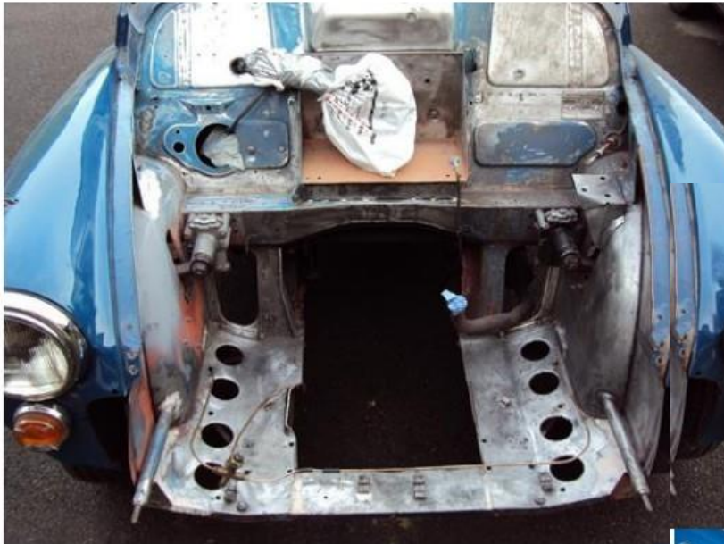
Engine is out and hours of scraping get the thick layers of sound deadening off the engine compartment.
