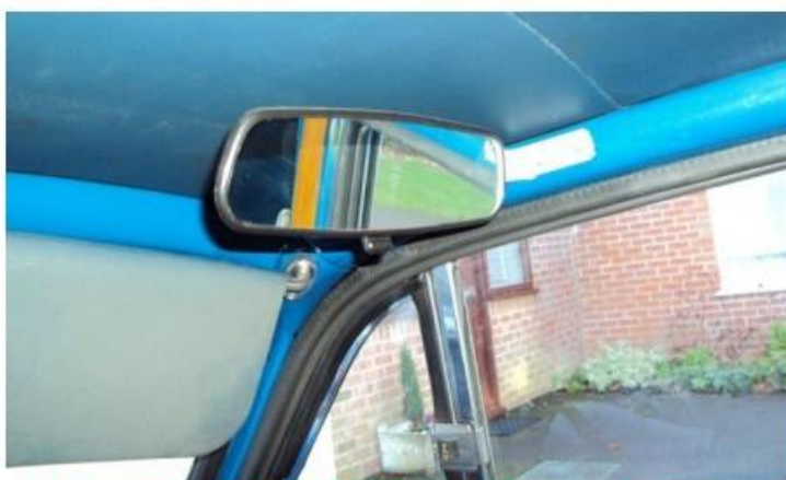
Rear views in a van are dreadful, even with big wing mirrors you can't see directly behind you. This mirror fitted to the door frame is offset enough to allow a view of traffic directly behind.
