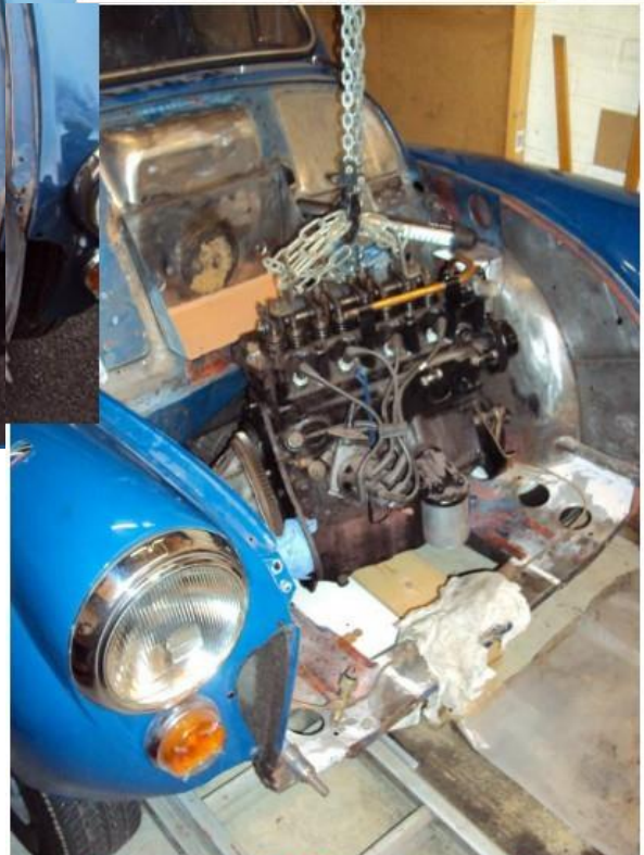
Out comes the 1098cc engine ready for a Marina 1275cc to drop in.
